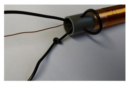
The next step is to drill two more holes as shown in the photo above. These holes will be used to put the wire through, which will be used as the strain relief. Finish this step by tying a knot in the wire and pulling it tight.
