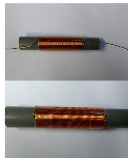
Try to wrap the coil as tight as possible, so there will not be any space left between the windings. Then fix the entire piece with some tape. Continue by drilling two small holes, right next to the coil, where you can stick the ends of the wire in.
