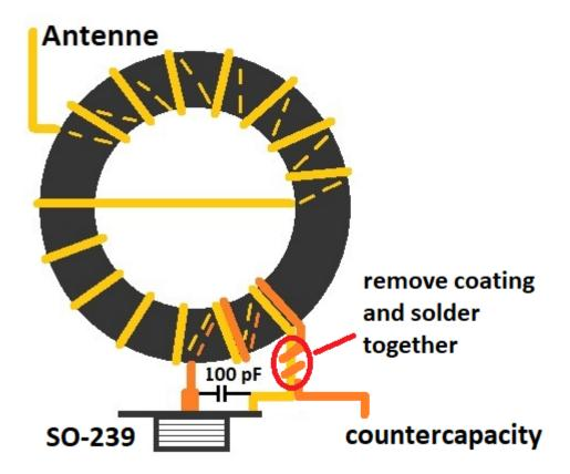
Fold about 20 cm of the enameled copper wire in half and lightly twist the first 15 cm to hold it together. Make sure to not twist the copper too much, because this might create strange effects in the transformer at a later point. Now take the point where the two pieces of wire become one and place this on the toroid. Now wrap the double part twice around the core. Then wrap the other 12 windings as shown in the pictures below. Cross over to the other side after the sixth wind.
