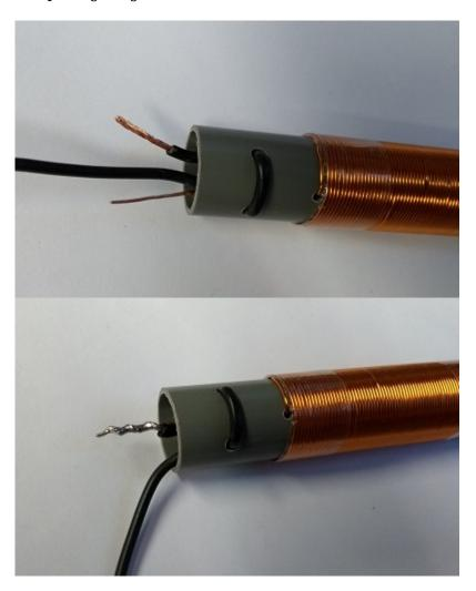
The excess wire can be cut off from the winding wire and the antenna wire. Leave just enough so there will be enough material for soldering. Make sure that the winding wire is completely stripped of the enamel layer. This can easily be done with a sharp knife or some sandpaper. Now solder the wire to the coil and put this into the pipe.
