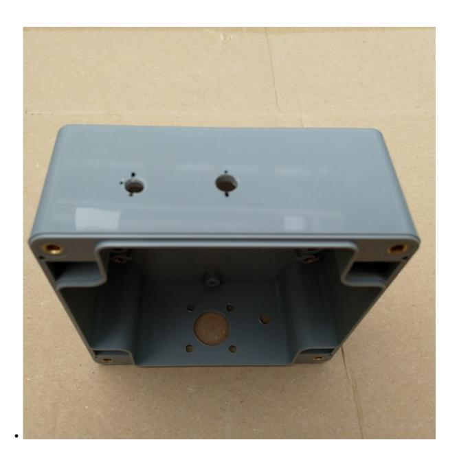
After drilling all the holes, we can find out if everything fits the way it should. Here you can see the result of drilling the holes and tightening the screws. When attaching the 5 mm bolts on the inside of the box, use two tooth-spring rings. One above and one below the cable lug, this will prevent it from rotating later when connecting the antenna wire or counter poise capacitance. Use a tan to pull the blue plastic part of the cable lug.
